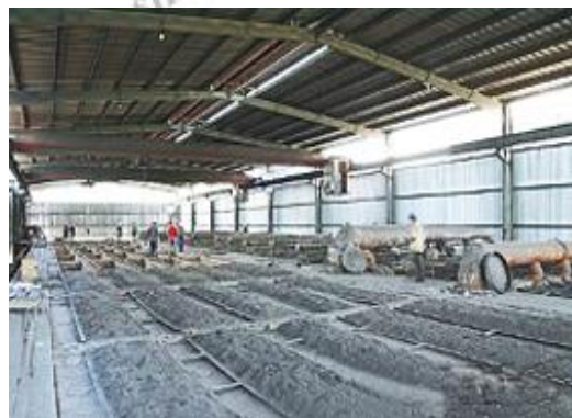
18-Room Ring Type Baking Furnace
